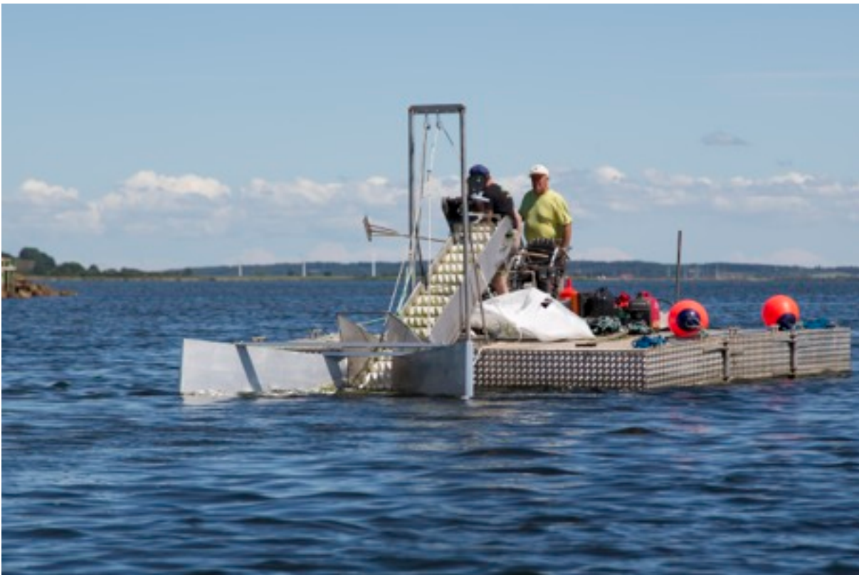
Figure 4. Automated seed harvester. Photo credits to Flemming Gertz.
